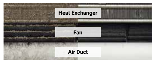
Without Dual Barrier Coating (After 10 Years) With Dual Barrier Coating
