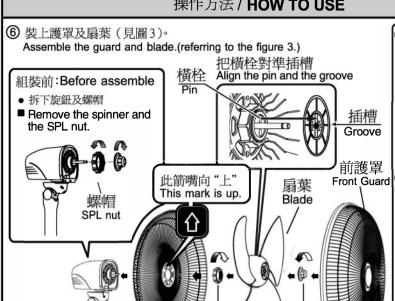
1 對準護罩上的標記 然後把前護置套上 Align with the mark on back guard and put two quards together.
