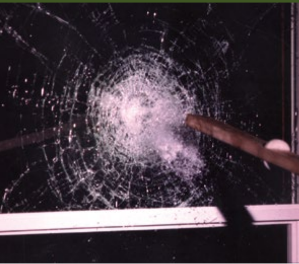
Glass Impact Testing at PGT's North Venice Production Facility
