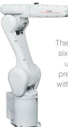
The vertically-articulated, six-axis robot increases uptime and enables predictive maintenance with integrated software.
