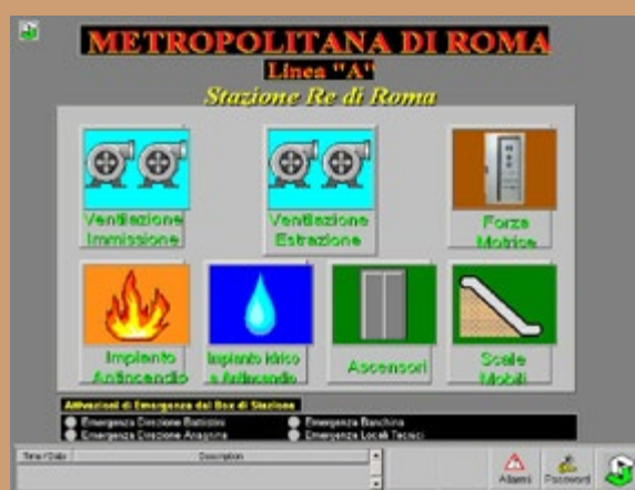
Station Overview Screen
