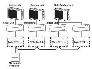
\*When using group control the MA controller must be connected to the lowest refrigerant address.
