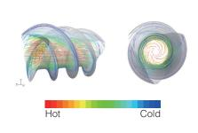
Using twist pipes as water pipes and running the refrigerant pipes along their grooves help increase the heat-conductive area, allowing for better heat transfer.
