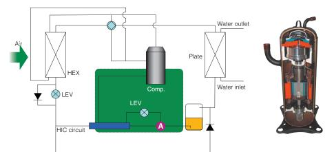
Two-phase refrigerant is separated into liquid refrigerant and gas refrigerant at point A.
