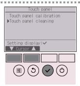
Move the cursor to "Touch panel cleaning" with the F1 or F2 button, and press the SELECT button.
