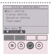
Move the cursor to "Basic setting" with the F1 or F2 button, and press the SELECT button.
