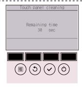
This screen allows the user to wipe the touch panel for 30 seconds without accidentally changing the settings.
