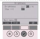
Adjust the brightness with the F1 or F2 button. "ON" or "OFF" can be selected for the "Stay lit" setting with the F4 button.
