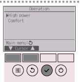
Select "High power" from the Operation menu during Cooling, Heating, or Auto operation, and press the SELECT button.
