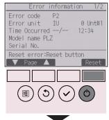
Press the F4 button or the ON/OFF button to reset the error that is occurring.
