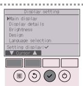
Move the cursor to "Main display" with the F1 or F2 button, and press the SELECT button.
