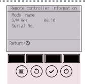
The model name, software version, and serial number of the remote controller in use can be checked.
