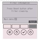
Press the F4 button to reset filter sign.
