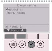
Move the cursor to "Restriction" with the F1 or F2 button, and press the SELECT button.
