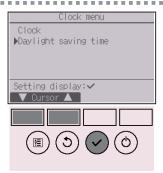
Move the cursor to "Daylight saving time" with the F1 or F2 button, and press the SELECT button.
