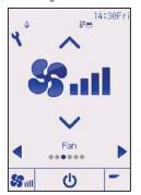
Each pressing of the  $\P$  or  $\blacktriangle$  button cycles through the following fan speeds.
