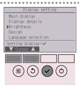
Move the cursor to "Brightness" with the F1 or F2 button, and press the SELECT button.
