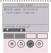
Move the cursor to "Touch panel calibration" with the F1 or F2 button, and press the SELECT button.
