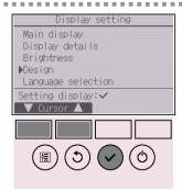
Move the cursor to "Design" with the F1 or F2 button, and press the SELECT button.
