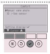
Select "Manual vane angle" with the F1 or F2 button, and press the SELECT button.
