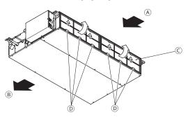
While lifting the filter knob, pull it.
