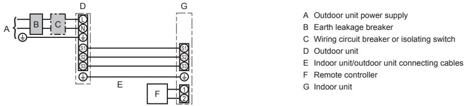
\* Affix label A that is included with the manuals near each wiring diagram for the indoor and outdoor units.
