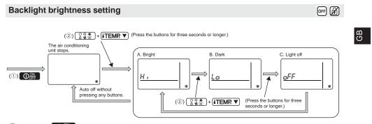
1 Press the  $\bigcirc_{OFF}^{ON}$  button to stop the air conditioning unit.
