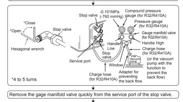
After refrigerant pipes are connected and evacuated, fully open all stop valves on gas and liquid pipe sides.
