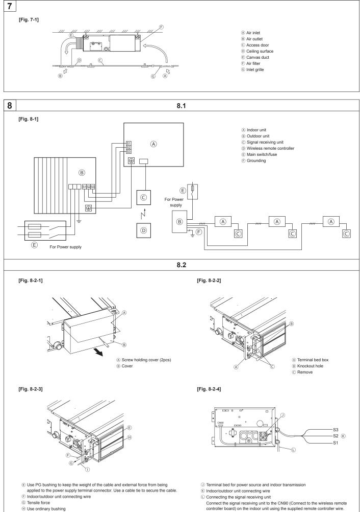
① Signal receiving unit wiring
