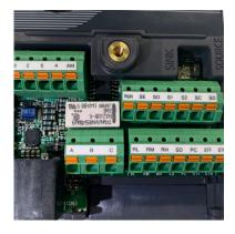
**Easy Wiring** With the integrated spring clamp terminals to connect control and power lines, the wiring became easier and more secure.
