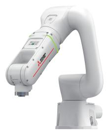
Mitsubishi Electric MELFA ASSISTA Cobot with advanced safety technology can share a workplace with humans without the need of guard or safety fences. The setup of the robot is easy even without specialised knowledge of robots. Typical applications include assembly tasks, packing operations, precise holding or repetitive pick and place. Simpler, easier and more flexible, this robot will change your perception of what a "robot" is.
