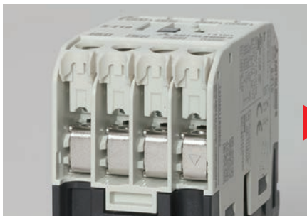
① Screw holder lifts up the screw.
