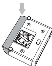
9. Tighten up the screw (a) using a Phillips screwdriver (+) to secure the lamp cover.
