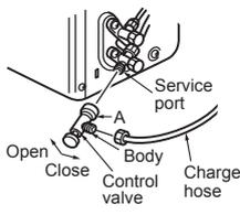
When attaching the control valve to the service port, valve core may deform or loosen if excess pressure is applied. This may cause gas leak.
