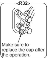
Make sure to replace the cap after the operation.
