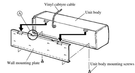
Remove the two mounting screws from the unit body, then remove the wall mounting plate from the unit body.
