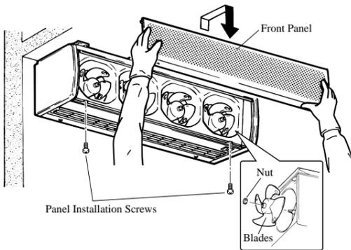
1. Take out the two screws used to install the front panel.
