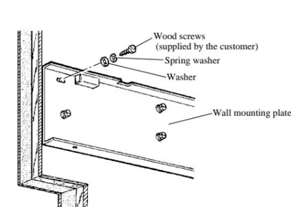
If the panel thickness is 20 mm or greater, mount the wall mounting plate directly on the wall with the washers and spring washers supplied with the air curtain, and wood screws (supplied by the customer). If the panel thickness is less than 20 mm, install a reinforcing board (supplied by the customer) so that the total thickness becomes 20 mm or greater.
