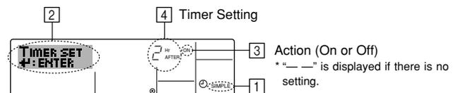
1. Be sure that you are at a standard control screen, and that the simple timer indicator is visible in the display (at ①).
