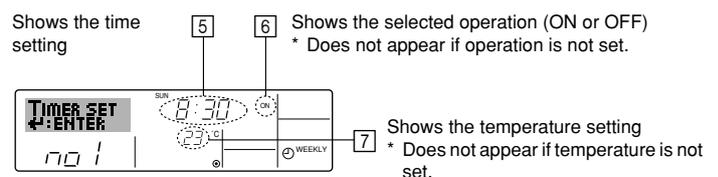
5. Press the appropriate Set Time button ⑩ as necessary to set the desired time (at ⑤).
