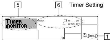
1. Be sure that the simple timer indicator is visible on the screen (at 1).
