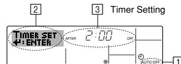
1. Be sure that you are at a standard control screen, and that the Auto Off timer indicator is visible in the display (at 1). When something other than the Auto Off Timer is displayed, set it to AUTO OFF TIMER using the function selection of remote controller (see 8.[4]-3 (3)) timer function setting.
