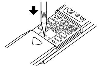
Press the Reset button with an object that has a narrow end.
